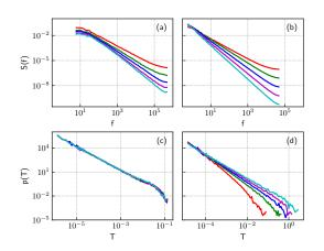
Time series from ABM and fBm, PSDs of which are similar, compare (a) and (b). As we can see their burst duration PDFs differ, compare (c) and (d).
