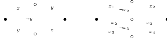
Fig. 1.5 A nondeterministic branching program computing the majority function \text{Maj}_3(x, y, z) = 1 iff x + y + z \geq 2 , and a non-monotone switching network computing the threshold function \text{Th}_2^4(x_1, x_2, x_3, x_4) = 1 iff x_1 + x_2 + x_3 + x_4 \geq 2 .
