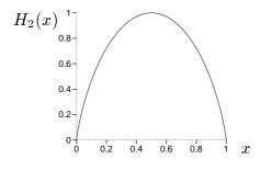
FIGURE 1. The binary entropy function  $H_2(x) = -x \log_2 x - (1-x) \log_2(1-x)$ .
