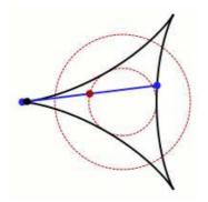
FIGURE 1. As the middle (flexible) point moves around the smaller circle, the needle rotates through  $360^{\circ}$ .
