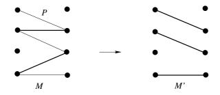
FIGURE 2. Enlarging the matching M by the M-augmenting path P
