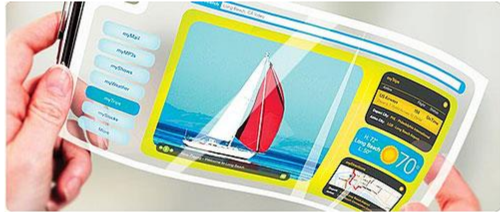
Flexible organic light-emitting diode
