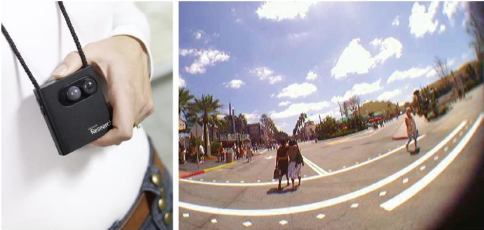
Figure 3.5 The SenseCam device and a digital image taken with it Source: ©Microsoft Research Cambridge.
