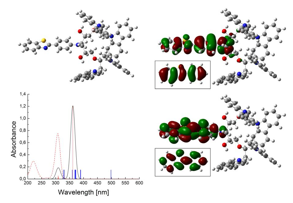
*Left:* molecular structure (*top*) and electronic excitations of 4-carbazole pbt ligand: singlet states (thin lines), triplet states (thick lines), theoretical absorption spectrum (solid line) and spectrum of pbt (dashed line). *Right:* HOMO (top) and LUMO (bottom) orbitals of pbt ligand (boxes) and 4-carbazole pbt ligand
