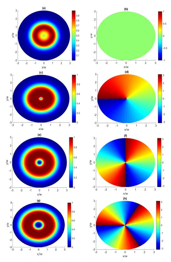
**Figure 2.** Intensity distributions in arbitrary units (**a**,**c**,**e**,**g**) and the corresponding phase patterns (**b**,**d**,**f**,**h**) of generated FWM light for different OAM numbers  $l_c = 0, 1, 2, 3$ . The selected parameters are given by  $\Omega_d = 0.10\gamma_{30}$ ,  $\Delta_p = \Delta_s = 0$ ,  $\gamma_{10} = \gamma_{30}$ ,  $\gamma_{20} = 0.02\gamma_{30}$ ,  $\gamma_{40} = 0.001\gamma_{30}$ , k = 0.29,  $\Omega_s = 2.5\gamma_{30}$ , and  $\varepsilon_c = 4\gamma_{30}$ .
