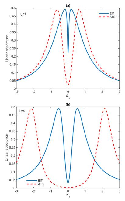
**Figure 4.** Linear absorption of the FWM light  $\text{Im}(\sigma_{30}^{(1)})$  vs. probe detuning when the coupling light carries an optical vortex (**a**)  $l_c = 1$  and (**b**)  $l_c = 4$ . The solid line corresponds to EIT ( $\varepsilon_c = 0.98\gamma_{30}$ ) and dashed line corresponds to ATS ( $\varepsilon_c = 4\gamma_{30}$ ). The selected parameters are r/w = 1.5,  $\gamma_{20} = 0.02\gamma_{30}$ .
