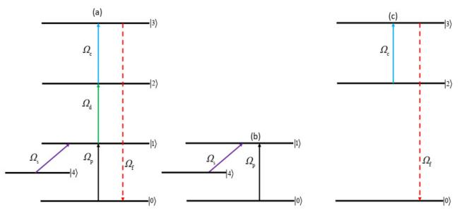
**Figure 1.** (a) A five-level quantum system interacting with probe and control fields. (b,c) Left and right  $\Lambda$  subsystems.
