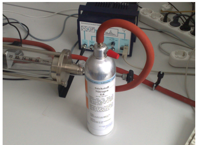
Fig. 13. Connecting the compressed gas cylinder to the fine control valve
