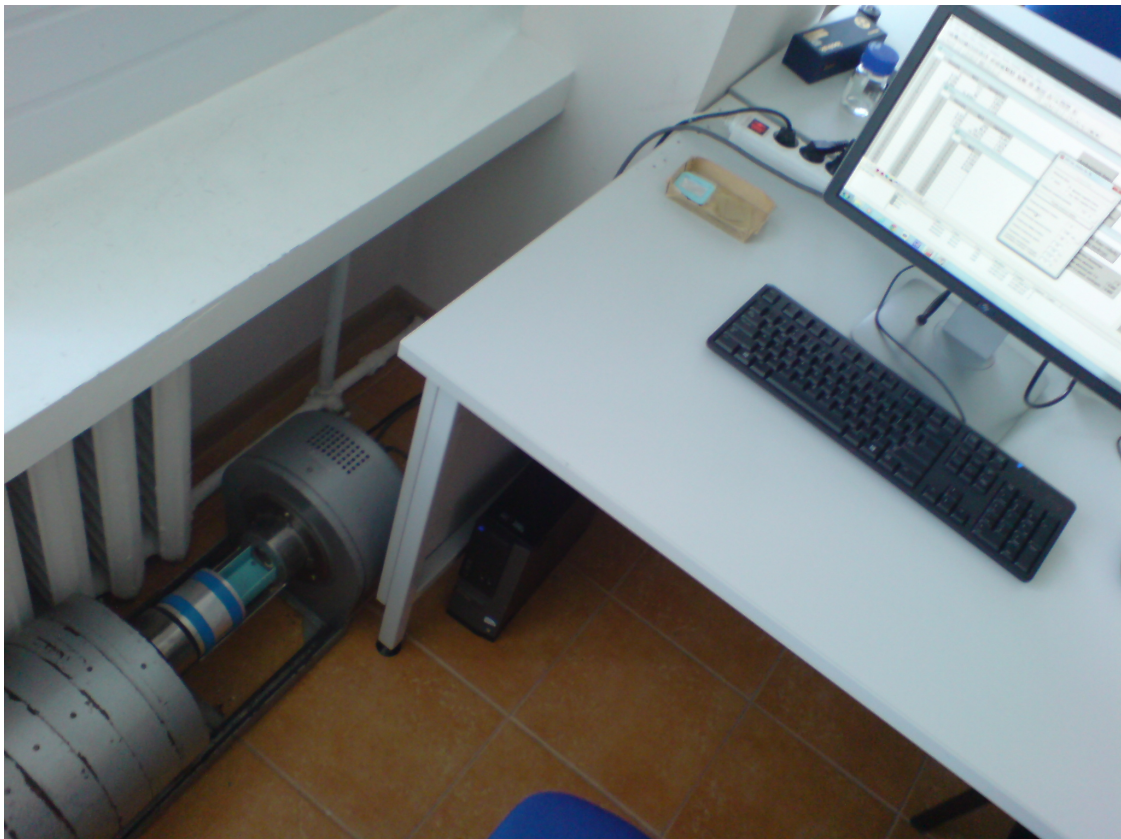
Fig. 9. A general view of the equipment for measuring absorption of beta particles. The detector device (UMF) is on the floor beside the table. An aluminum container with the radioactive material is placed in front of the detector. A box with aluminum and organic glass absorbers is visible on the table, as well as a monitor showing the main window of the control program and worksheets of the data analysis program “Origin” with measurement data.
