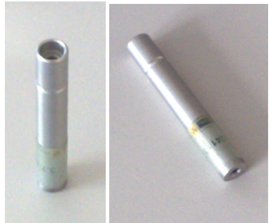
Fig. 7. The unsealed Am-241 source (the radioactive material is at the top)
