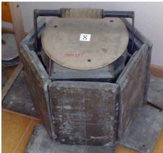
**Fig. 16.** The container of the neutron source (the source is at the bottom of the container). The container is surrounded by lead bricks that serve to decrease intensity of gamma radiation in the environment
