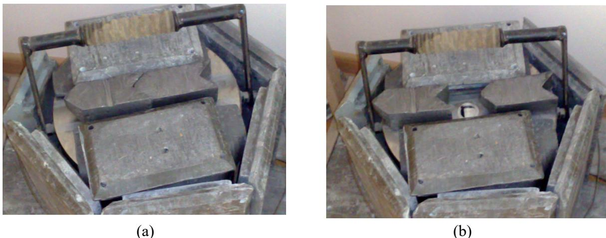
**Fig. 22.** The container of the neutron source: (a) without the lid; (b) with the sample slit uncovered
