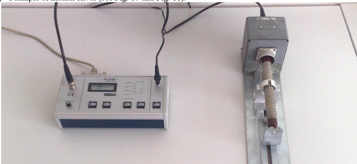
**Fig. 15.** The main components of the measuring equipment – **Isotrak** ratemeter (on the left) and Geiger-Müller counter (on the right). The counter is the metal tube. Near its center there is the sample holder, which ensures that the position of the sample relative to the detector is the same during all measurements (also see Fig. 18). The **Isotrak** ratemeter is connected with the detector and with the PC
